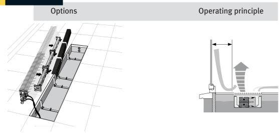
Flexible connections for fast assembly. Makes the Low- $H_2O$  heat exchanger removable for maintenance.
